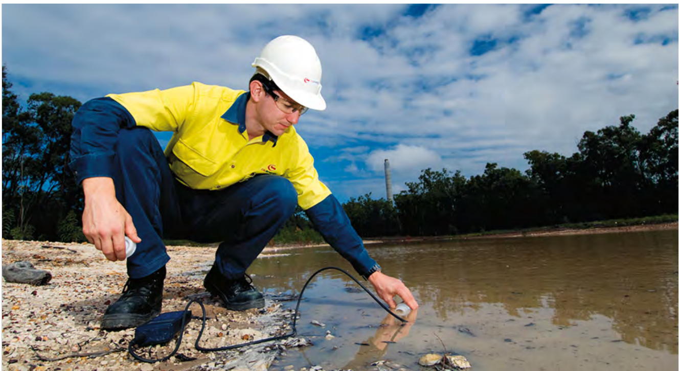
Kogan Creek Environmental and Industrial Chemist, Ian Richardson, regularly tests water quality as part of an ongoing environmental monitoring programme.
